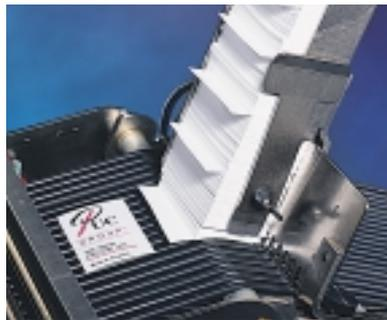
With economy in mind, the 676 offers the option of ink-save on one printhead, so that you can add spot colours without wasting ink! Like all Paxar electronic printers, the 676 is designed with ease of handling in mind and comes complete with the facility to cut printed labels, separate them into batches and stack them, ready to be sewn into your garments. The new Microstacker gives you the further option of producing labels down to 16mm x 32mm, ideal for intimate apparel and size tabs.
